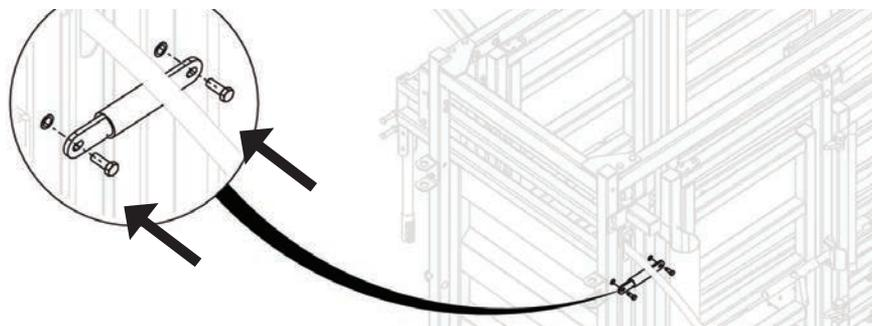
**7** Remove the rolling door lock and move to the opposite side.
